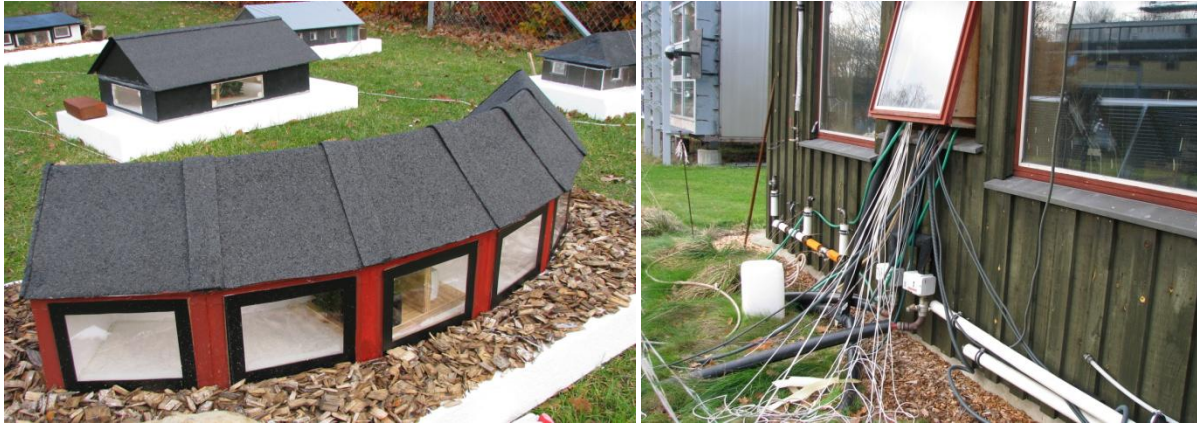
Figure 6. The operating phase, where the students test the houses outdoors – left. The houses are connected to the electrical power – right.
