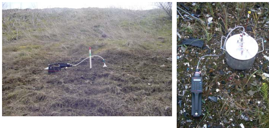
Figure 7. Hot spot on soil cover. In many cases a change in vegetation, or lack of vegetation has been observed at these zones of high landfill gas emission. The picture on the right shows the flux chamber coupled with the FID
