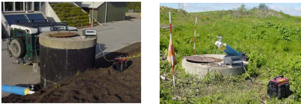
Figure 10. Methane emission measurements from leachate wells.
