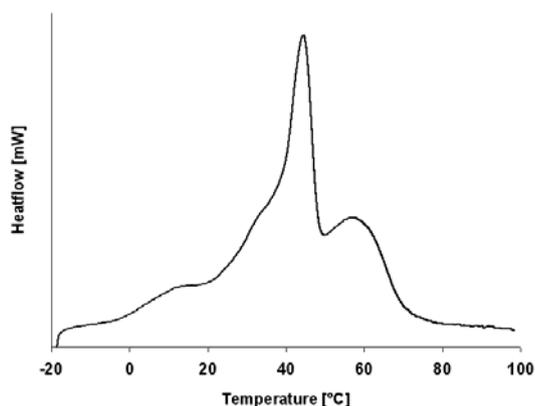
**Figure 2.** Thermal transitions of wheat straw wax determined by DSC.
