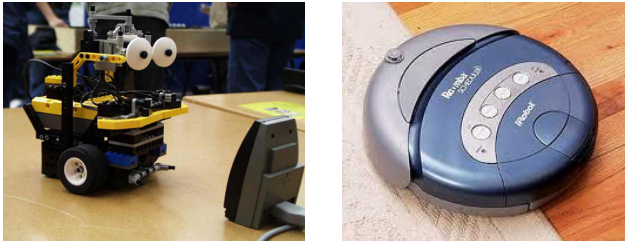
Fig. 8. left: RoboCupJunior, and right: Roomba, two examples of behavior-based robotics application.
