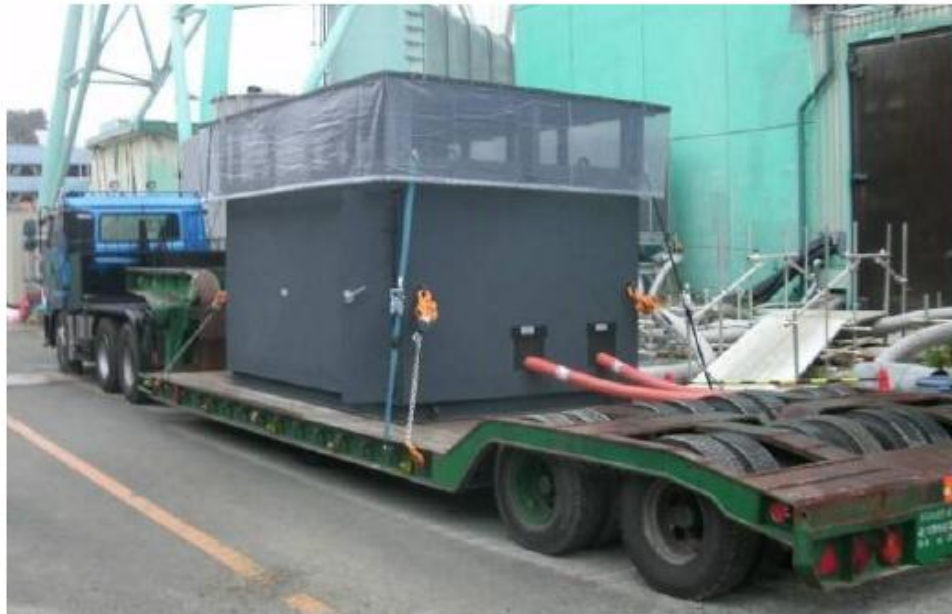
Figure 4: Caesium absorption apparatus inside shielding container
