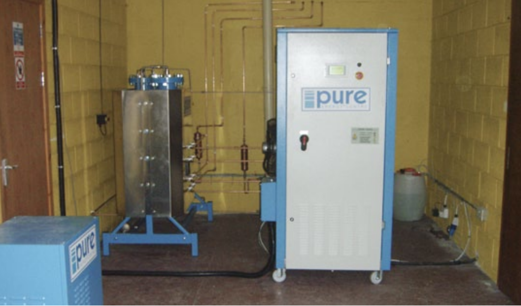
▲ Pure® Hydrogen production system
