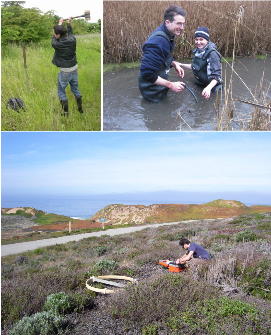
Figure 3.1 Installing a benchmark point for a geodesy survey at Risby Landfill (upper left). Seepage meter measurements at Risby Landfill (upper right). Performing a Time Domain Electromagnetic (TDEM) sounding at Monterey Bay, California (bottom).
