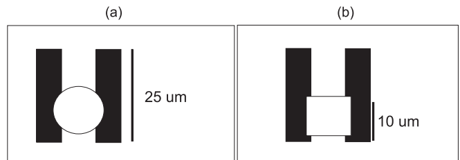
FIG. 4: (a) Cross section of a cell trap with a spherical cell (b) Cross section of a cell trap with an assumed cubic cell trapped
