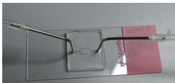
Figure 3.22: Fully assembled microFISH device with interconnects and tubings to connect it to the syringe pump.
