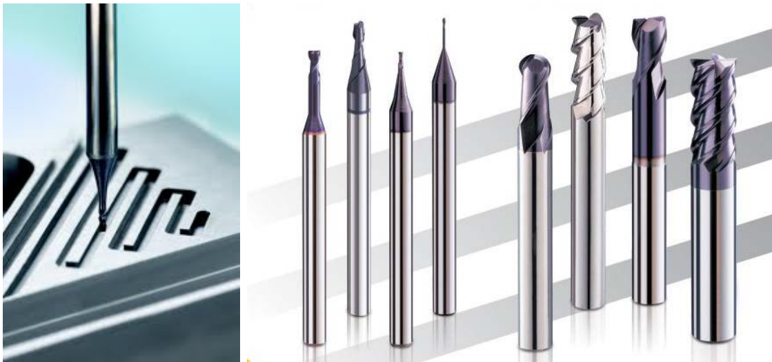
Figure 5.1: (Left) Micromilling process (Right) Tools used for micro milling (Courtesy: Janpo)
