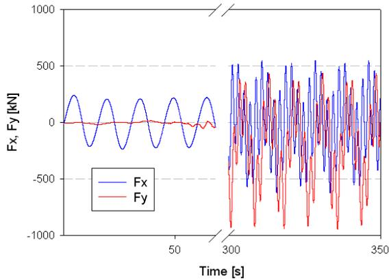
**Figure 17**  $F_x$ ,  $F_y$  on the tower section 15m above the sea. First time series (20-60s) with no rotation of the rotor, second time series (300-350s) at rated conditions
