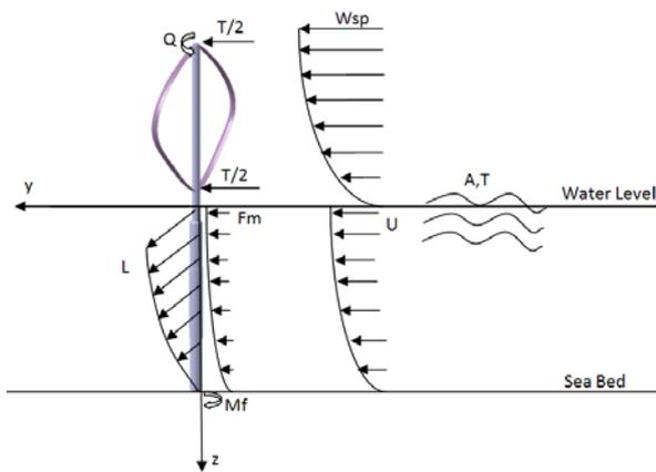
**Figure 5 External conditions and main loads on the turbine**
