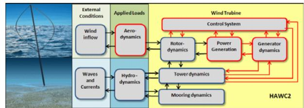
**Figure 6 Flow diagram of the HAWC2 code, in red the parts needing to be partially modified or added.**
