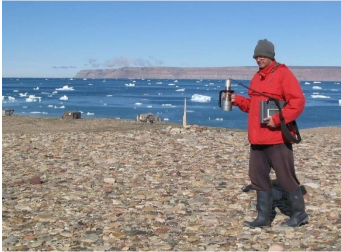
Figure 15. Portable gamma spectrometer for field measurement of ^{241}\text{Am} with detector at 1 m above ground.
