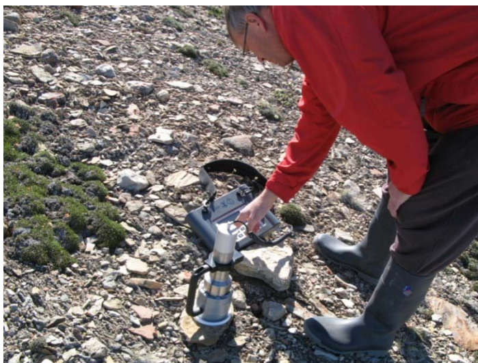
Figure 14. Portable gamma spectrometer for field measurement of ^{241}\text{Am} with detector placed on ground.
