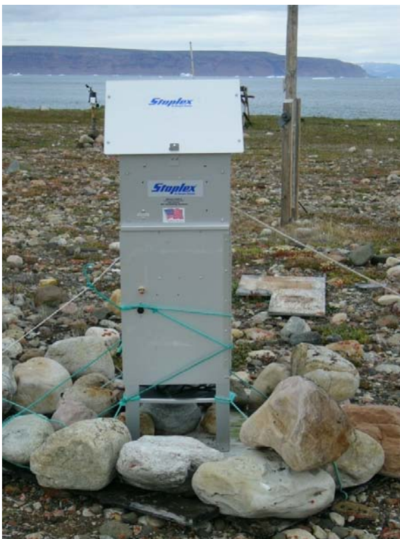
Figure 3. Air sampler at Narsaarsuk
