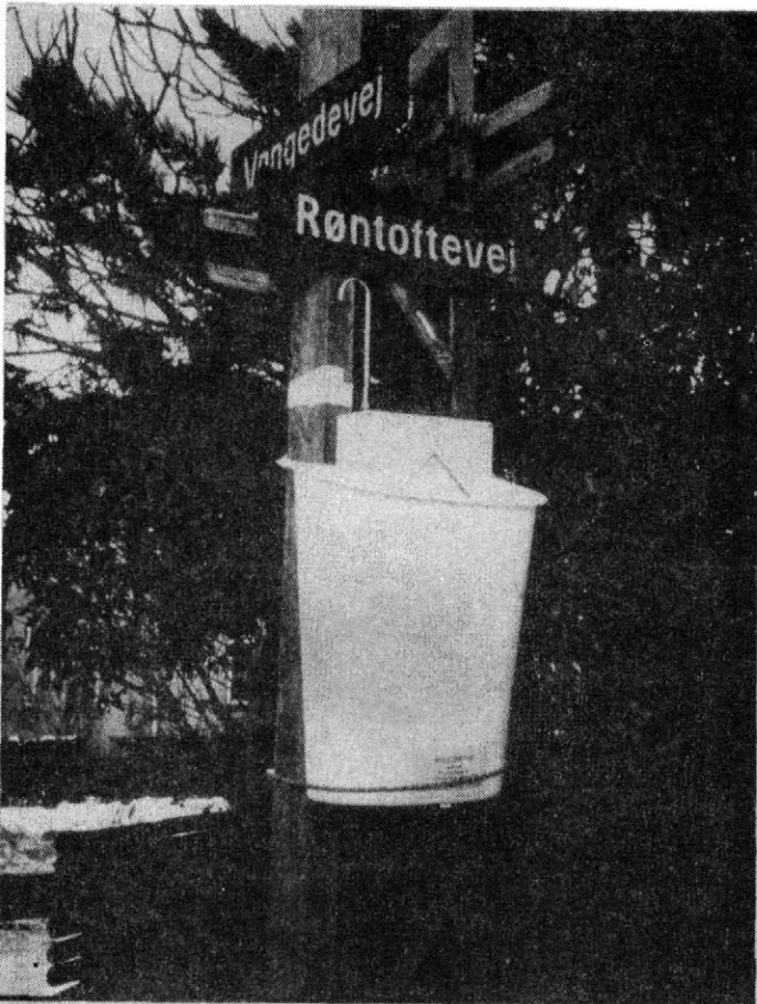
Fig. 5.8. Sampling unit mounted in lamppost in Copenhagen, ready for an experiment. The basket protects the Saran bags.
