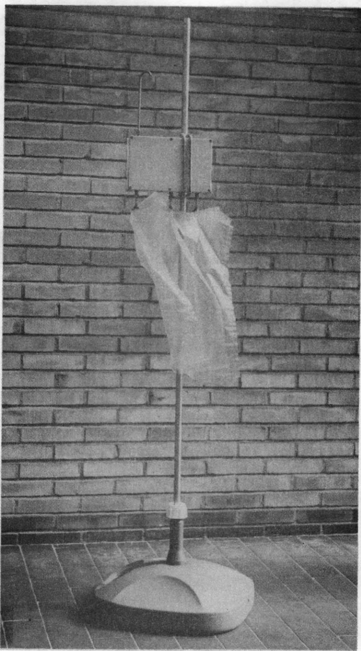
Fig. 5.7. Sampling unit mounted with plastic bags and placed on a portable rack.
