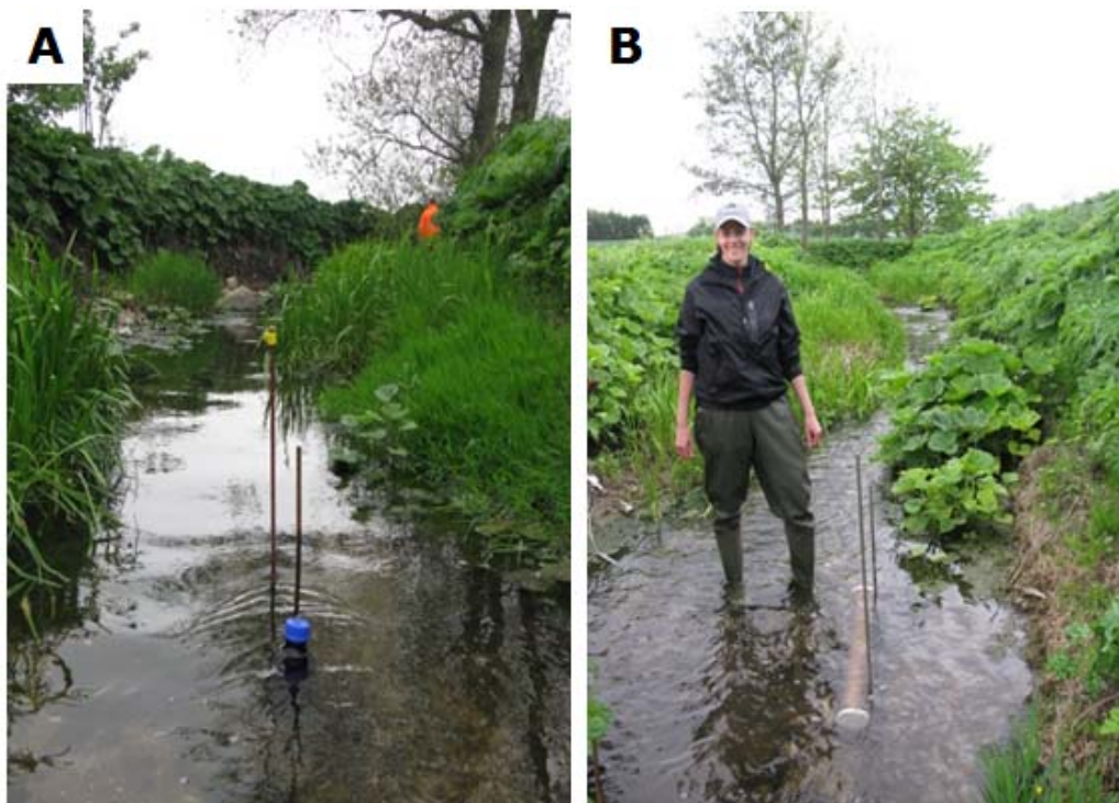
Figure 2: Photos from the field sampling in Skensved stream for the (a) event-controlled (storm-flow) runoff sampling system and (b) streambed sediment sampler.
