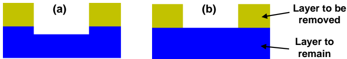
Figure 5.5: Illustration of the etching selectivity. (a) Poorly selective etch: removes the top layer, but also attacks the underlying material. (b) Highly selective etch: leaves the underlying material unharmed.
