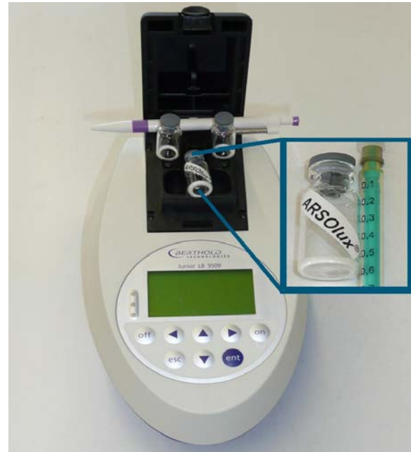
Figure 1. ARSOlux ® glass vials containing freeze dried bioreporter bacteria and portable luminometer for arsenic measurement.
