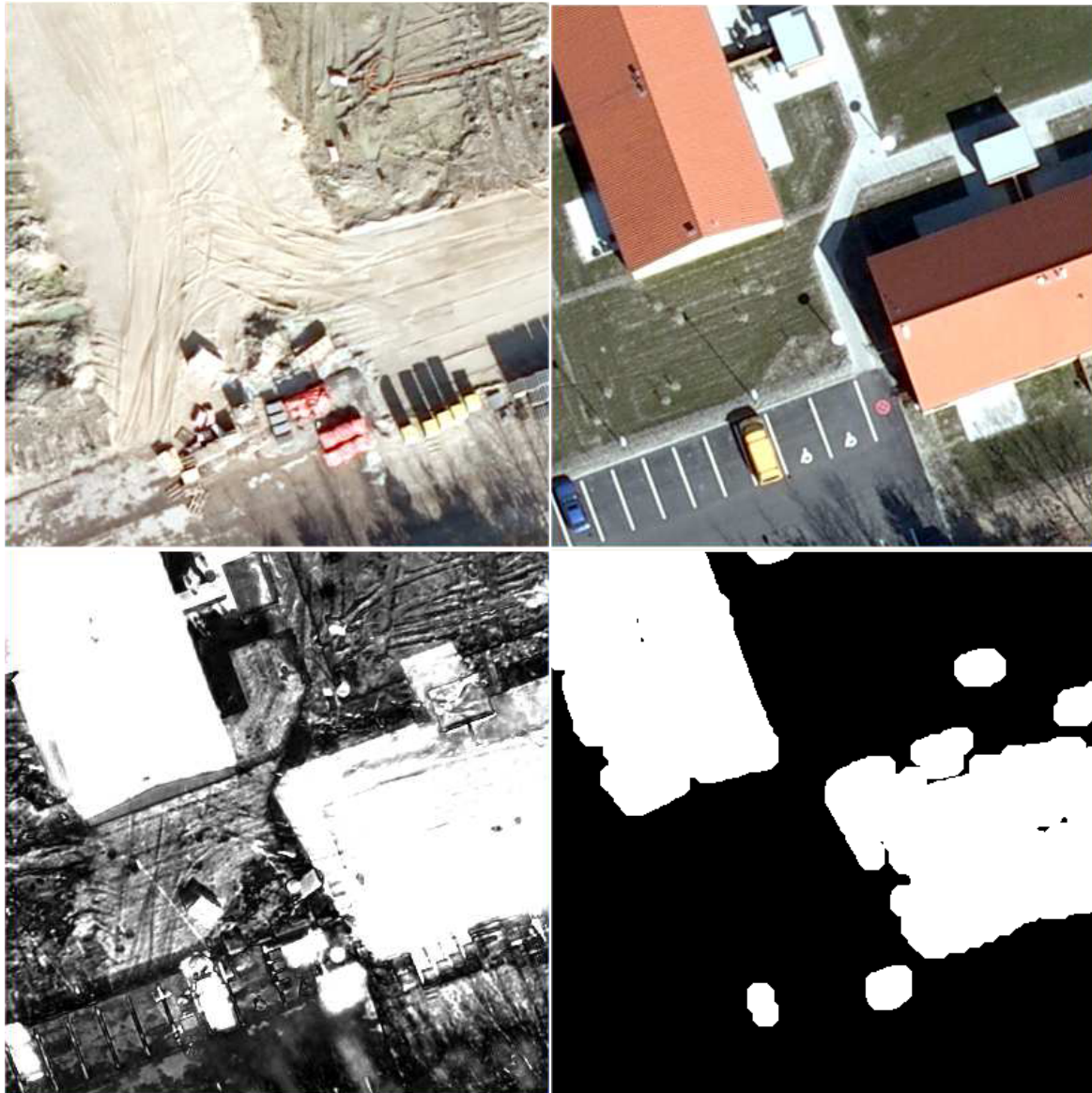
Figure 2: Results for the zoomed area from 6168_726. Changes between years 2007 and 2009. UL: Zoomed area from the 2007 scene. UR: Zoomed area from the 2009 scene. LL: Change image. LR: Significant change image
