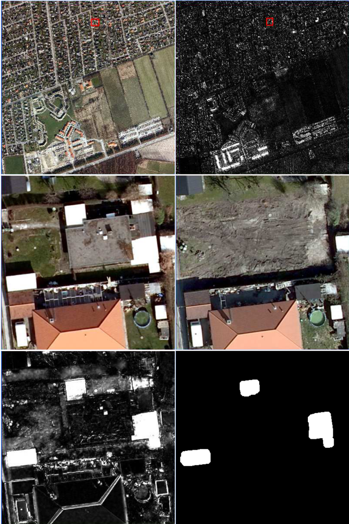
Figure 6: Example 4 for area from 6168_726. Changes between years 2007 and 2009. UL: The 2007 scene. UR: Change image. ML: Zoomed area from the 2007 scene. MR: Zoomed area from the 2009 scene. LL: Change image. LR: Significant change image.
