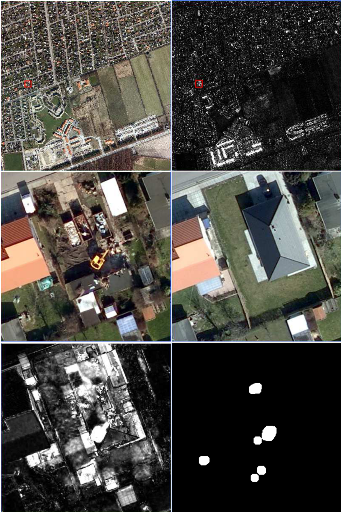
Figure 8: Example 6 for area from 6168_726. Changes between years 2007 and 2009. UL: The 2007 scene. UR: Change image. ML: Zoomed area from the 2007 scene. MR: Zoomed area from the 2009 scene. LL: Change image. LR: Significant change image.
