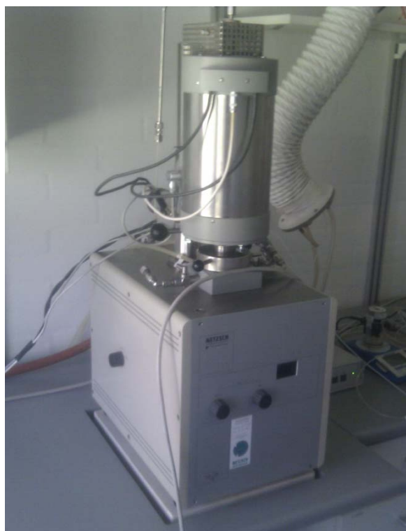
Figure 35 Netzsch 409C capable of doing TGA and DSC
