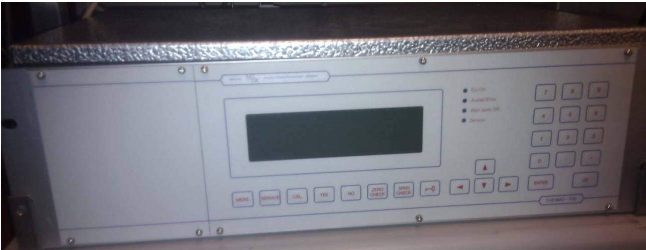
Figure 33 Picture of the Thermo FID produced by Mess & Analystechnik GmbH
