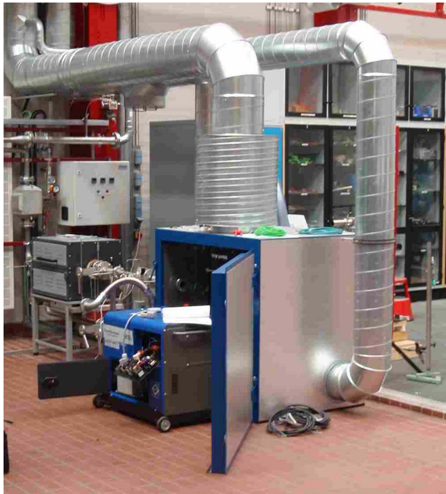
Figure 2: Diesel engine, noise reducing casing, cooling air pipes and oven with DPF inside.
