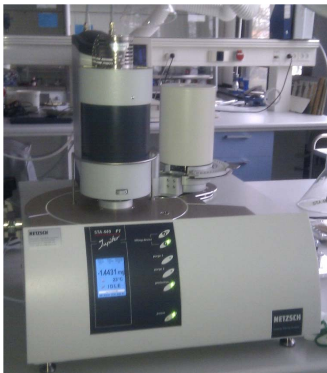
Figure 34 Netzsch 449FI Jupiter capable of doing TGA and DSC
