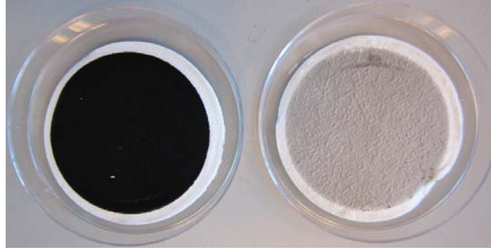
Figure 4: PM samples collected before and after DPF while running with DAKA biodiesel at 80 % load [2].
