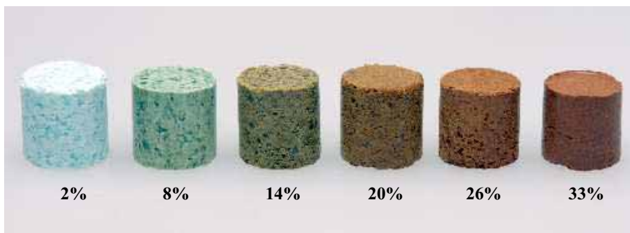
Figure 5-28: Picture of a pellet from each of the preparations in the Cu series. The figures indicate the Cu content of metals (Cu + Al).
