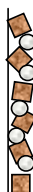
Figure 3-5: The single pellet string loading principle. Inert alumina or glass balls separate the individual catalyst pellets.
