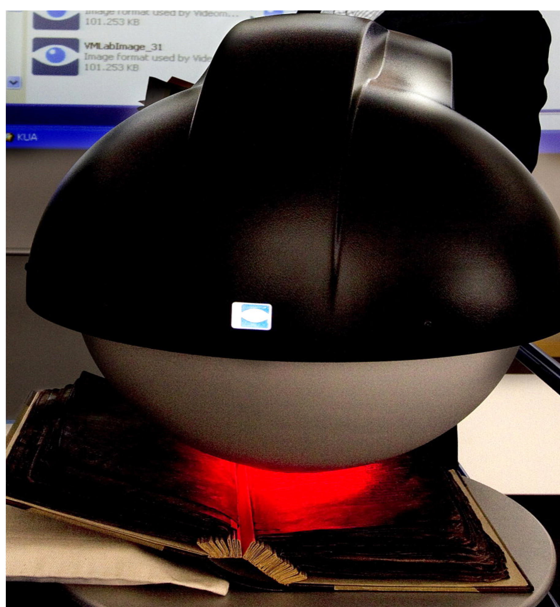
The sagas are scanned using VideometerLab, which produces multispectral images.
