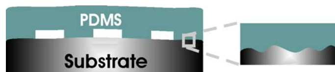
Figure 5 Conformal contact requires adaptation to height variations over long distances (left) and to small-scale roughness of the surface (right).
