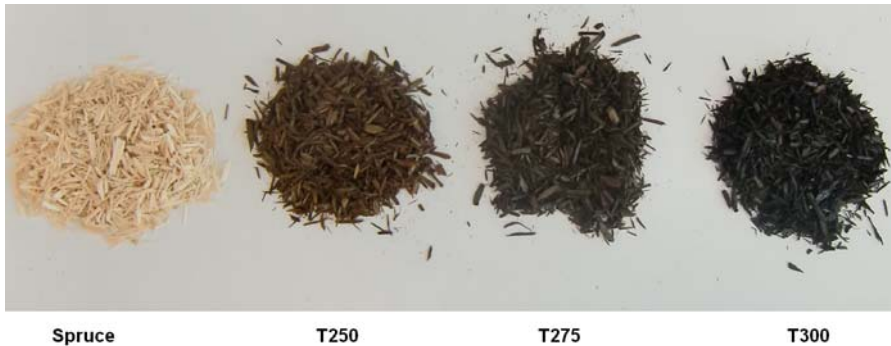
Figure 1. Color change during the torrefaction process.
