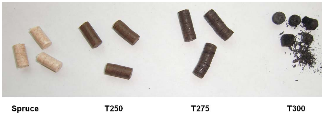
Figure 5. Pellets made from spruce and torrefied spruce. From left to right: Spruce and torrefied spruce at 250, 275 an 300 °C.
