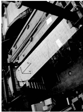
Figure 1 Wind turbine blade section under investigation with the coordinate system. For measurements of the original blade, axis system is rotated of 90° about z axis
