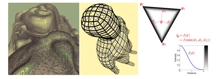
The standard procedure for wireframe drawing with hidden line removal on a graphics card has not changed for a long time: First the filled polygons are drawn, laying down the depth buffer. Next, the polygon edges are drawn as lines with a small depth offset to ensure that polygons do not occlude their own edges.
