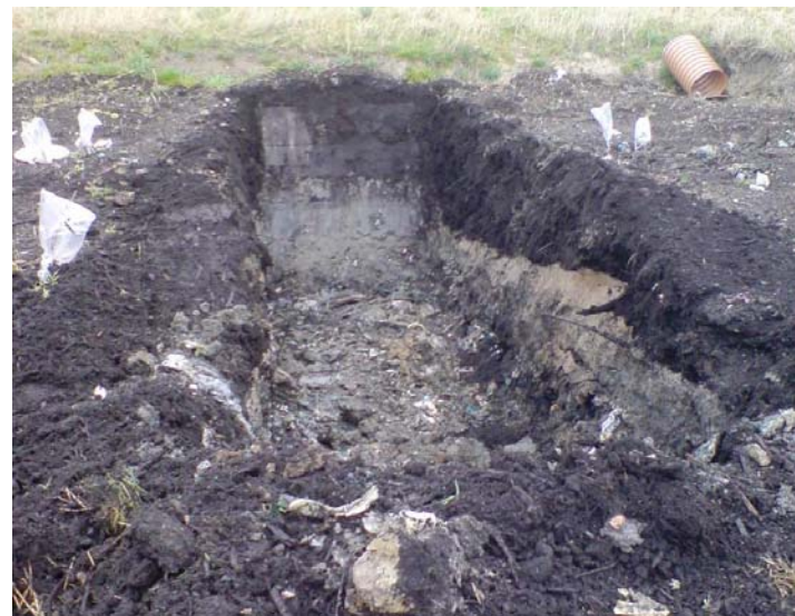
Figure 3.3. Excavation of window 1.4. The impermeable clay can clearly be seen in this picture. Furthermore it can be seen how the waste is mixed with clay and it can be seen how close the measuring stations are to the trench.
