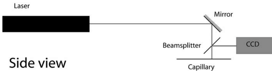
Figure 51. The micro interferometric backscatter detection setup used to monitor the binding events inside the capillary. The beamsplitter makes it possible to detect the centroid and the first fringes.
