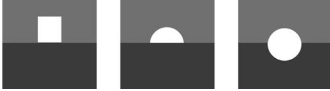
Figure 17. The three modeled geometries is drawn. The top part is modeled as being PDMS and the bottom part is modeled as glass. The cross-sectional area of the rectangular and the semicircular structure are also kept the same, thereby a direct comparison has been possible.
