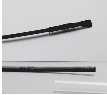
Figure 3.5: Photograph of the large RL/OSL fiber. Top: fiber 01, with shrinkflex wrapping. Bottom: fiber 43 using NOA 61 adhesive and an Araldite coating.
