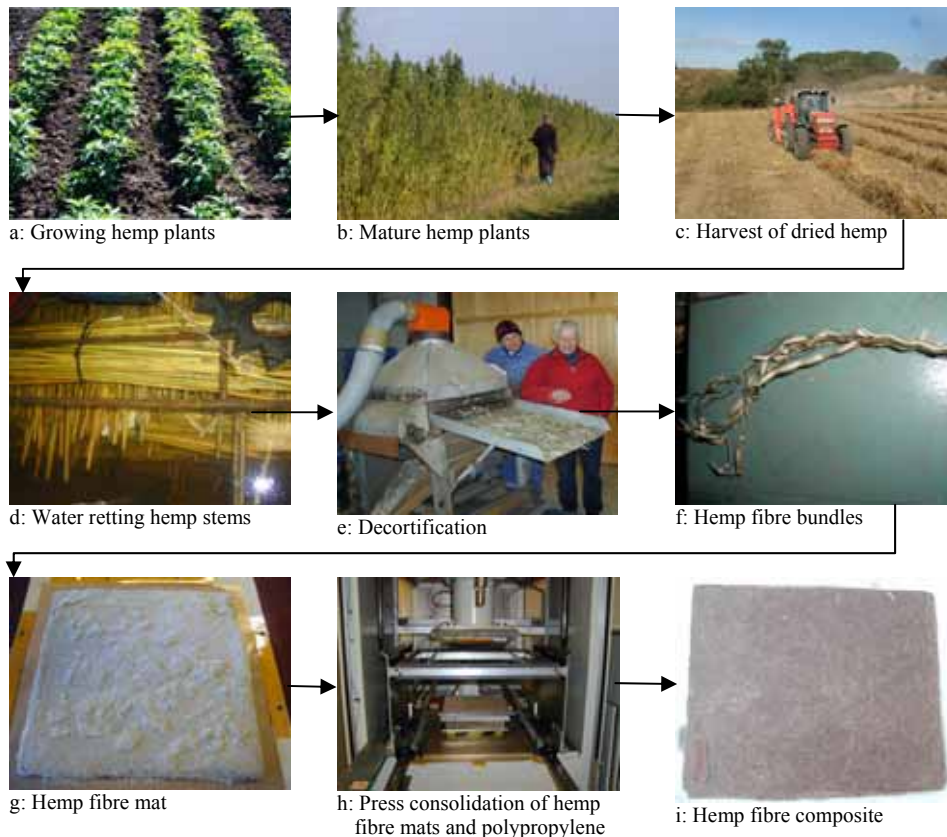
Figure 16. Traditional procedure for going from the hemp plant to fibre reinforced composite materials. The process goes through field cultivation (a → c), retting and decortification (d → f) and addition of polypropylene, heat and press consolidation (g → i).
