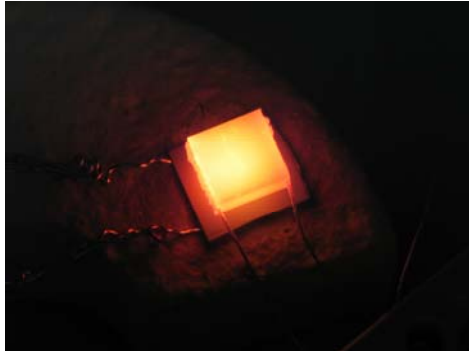
Figure 88. Photo of the (\text{ZrO}_2)_{0.97}(\text{Y}_2\text{O}_3)_{0.03} (10x10x3 mm) sample when heated with AC (10 kHz, 35 W).
