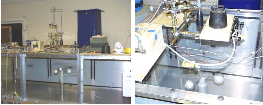
Figure 3-13 The pictures show the measurement setup for the measurement of torque from the Thies classical in LT5 2001. In the right picture the motor (black) and the thin shaft from the motor shaft to the hub of the anemometer rotor can be seen.
