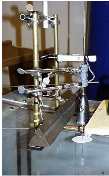
Figure 3-17 Torque measurement system with motor in torpedo like housing, bearings on spring loaded mounting rod in grey housing and spring balanced strain gauge bridge attached to the mounting rod to the left of the light grey attachment fixture
