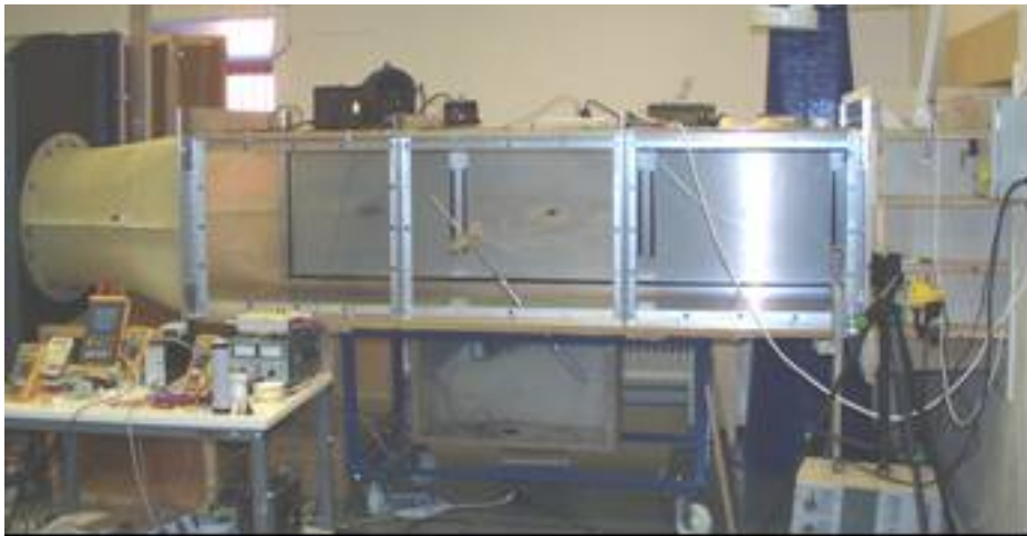
Figure 3-1 The large test section of LT5. The air is sucked from right to left and is blown out through a window in the back.
