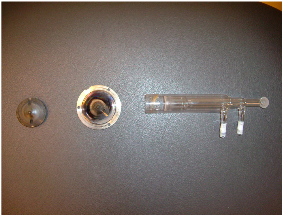
Figure 1 The torch and the two cones separating the plasma from the mass spectrometer.
