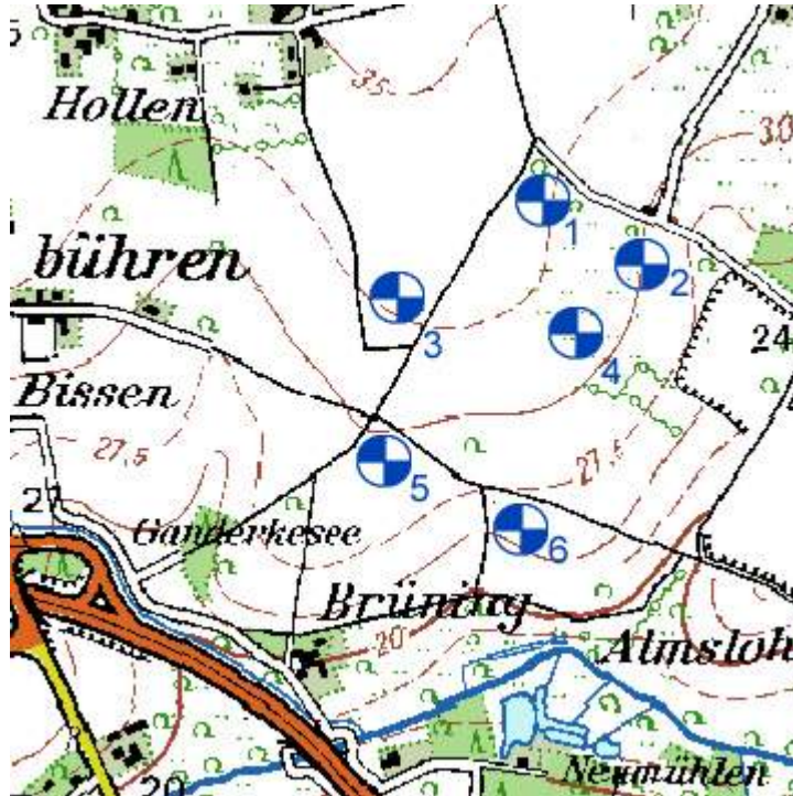
Figure 32: The layout of the Gruppenbühen wind farm. The motorway seen is the A1 west of Bremen.
