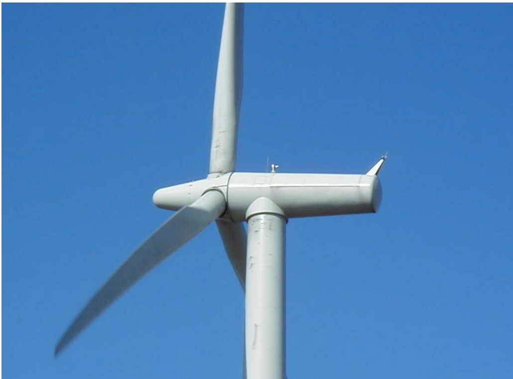
Figure 29: Turbine 7 with the video camera on top, as seen from the ground.
