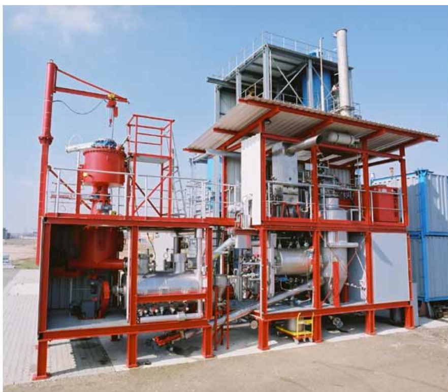
Figure 9. Small scale Gasifier Carbo compact, 150\text{ kW}_e , Picture courtesy of Technischer Apparatebau Freiberg
