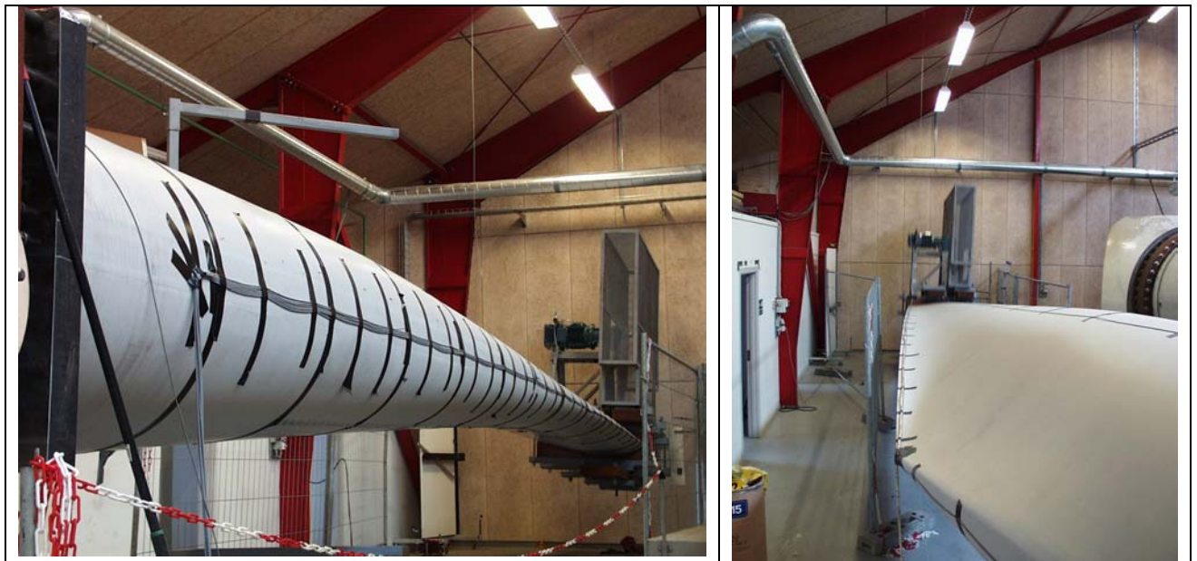
Figure 10. Test configuration at the flapwise fatigue test.
