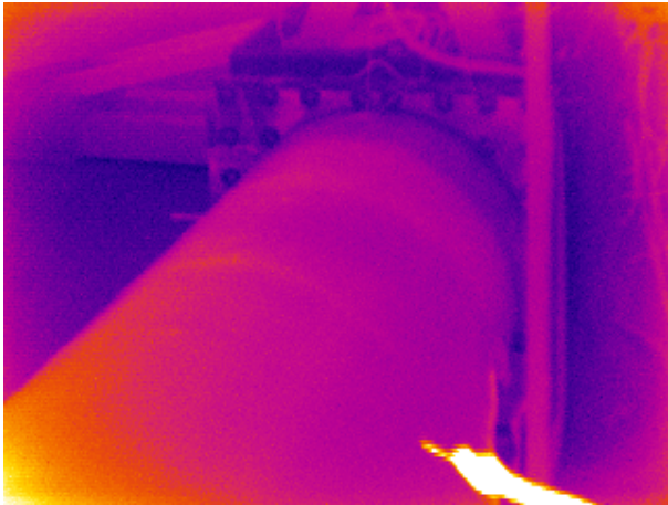
Figure 13. Thermal image of upwind side of root section
