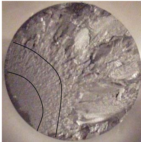
Figure 3-1 Fracture surface on test specimen with crack initiation (left), initial fracture (middle) and final fracture (right) areas.
