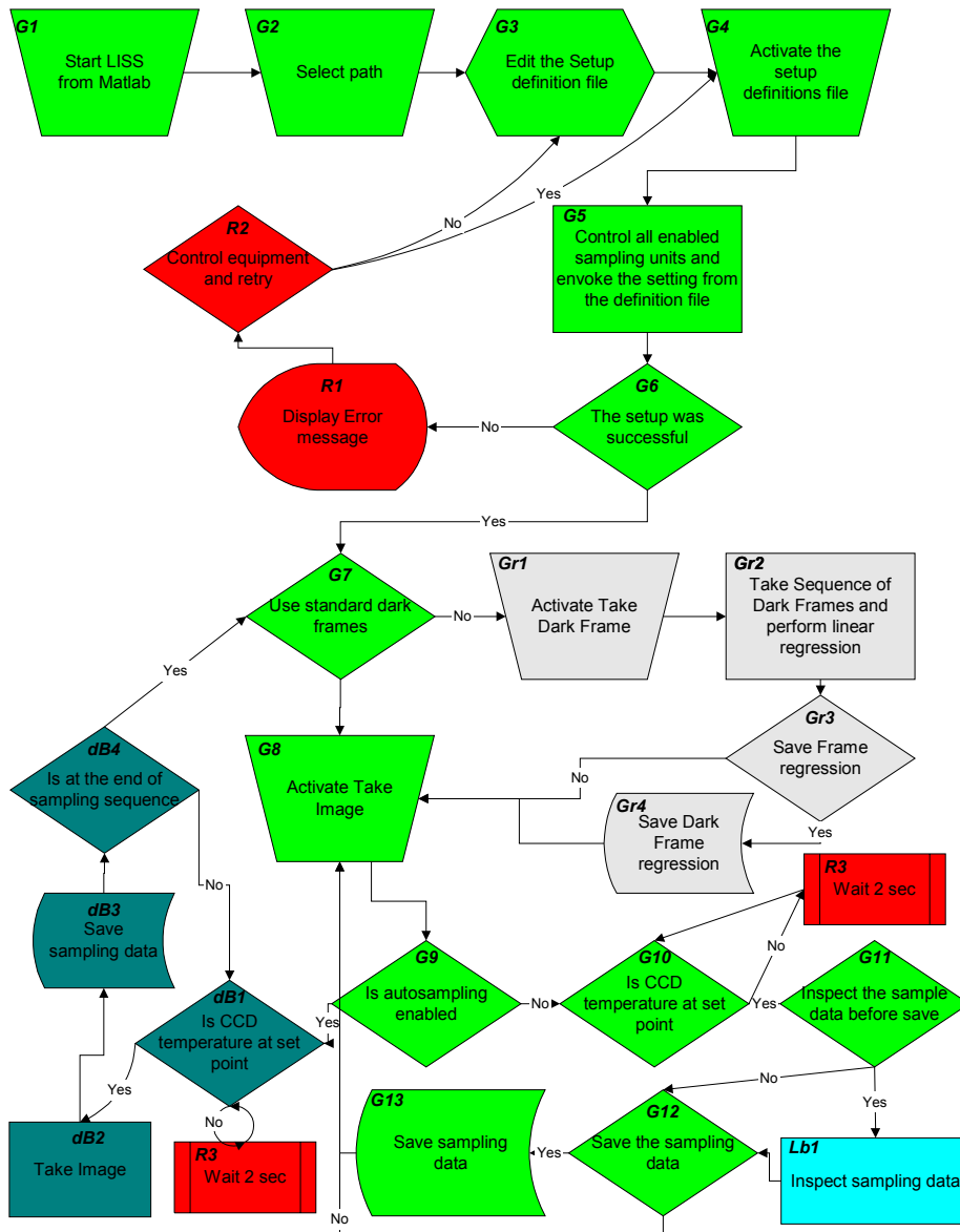
Figure 5: Flow chart illustrates the decisions and flow of action during a measuring session with the LISS software. The green colored boxes show normal flow of actions. The red boxes show when something goes wrong. The dark blue boxes illustrate automated sampling. The light grey boxes show the decisions needed concerning dark frames, and the light blue box illustrates the flow for performing manual inspection of data sampling before saving.
