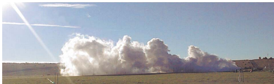
Experimental release of hydrogen fluoride (HF) within the URAHFREP EU project. It is tested whether cloud buoyancy, produced by a reaction between HF and atmospheric humidity, would be sufficient to lift the toxic plume off the ground.
