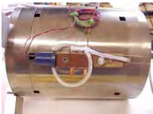
Fig. 1. Superconducting magnet in iron shielding with persistent switch mounted on the side. Dimensions \text{\O}240\text{mm} \times 280 mm. Weight = 50 kg.
