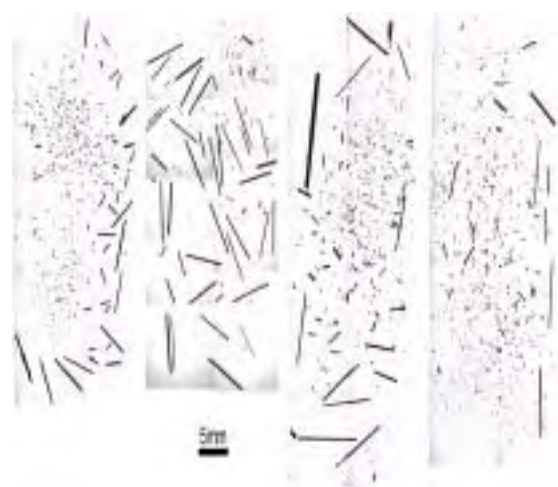
Fig. 2. Pieces of filaments after 1 min of ultrasonic vibration. Intermediate load from left to right: 0 kN, 3 kN, 17 kN, 29 kN.
