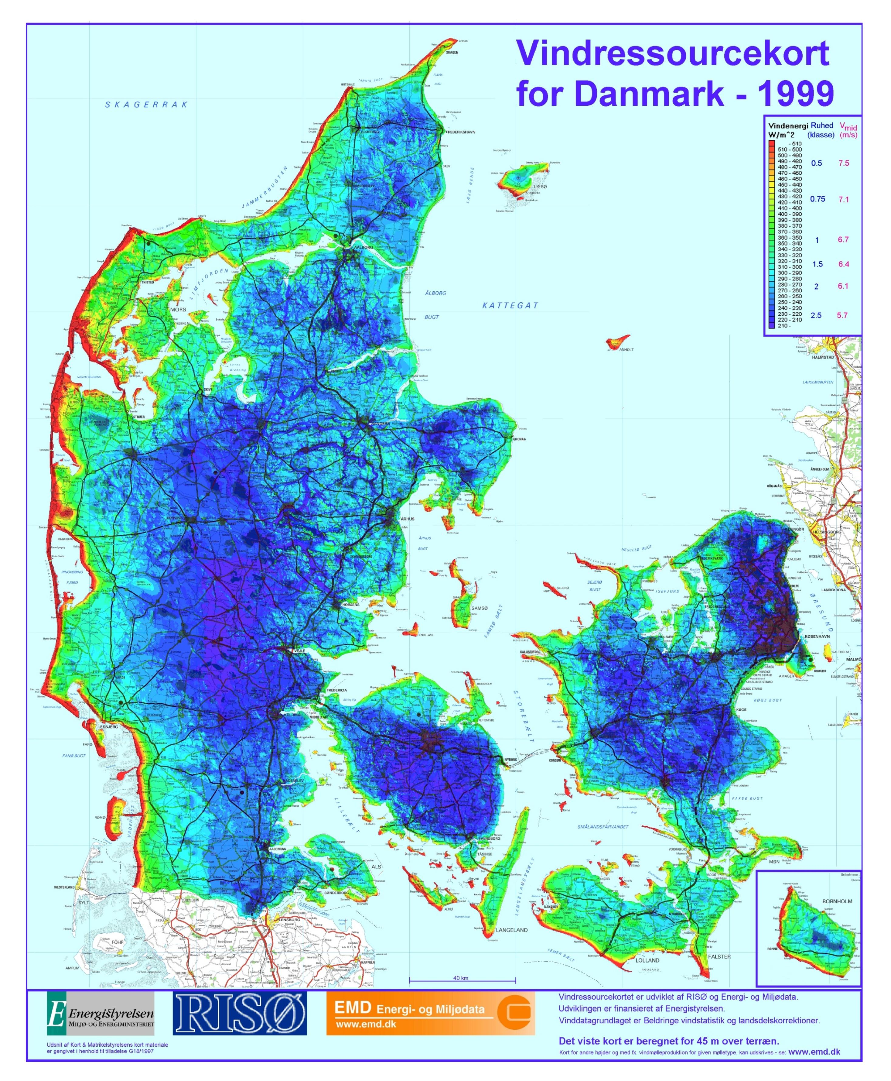
The WAsP program can be used to map the actual wind resource over large regions: The wind resource of Denmark (43,093 km<sup>2</sup>) is shown above – as the energy density [Wm<sup>-2</sup>] at a height of 45 m a.g.l. The methodology/verification is outlined in the paper and the wind resource map of Denmark can be downloaded from www.emd.dk.
