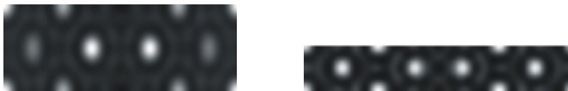
Fig. 1. Possible scattering potentials derived from the SXR in-plane data using direct methods: left, Cu 3 Au(110)-(4×1) and (b) Au 3 Cu(110)-(1×4). In both cases p2mm symmetry is assumed.
