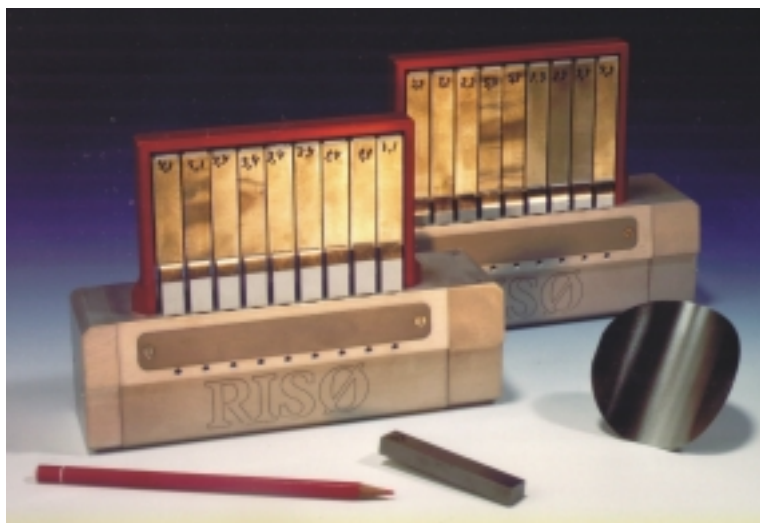
Fig. 1. The composite germanium wafer monochromators used at Risø and Kjeller since early 1997. The seven 20-wafer composite strips are mounted in the Risø design focusing monochromator holder, which are commercially available. The monochromator holder may be mounted for horizontal focusing (as shown) or for vertical focusing (normal monochromator).
