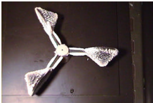
Figure 24. a) An example of rime accretion upon a WAA unheated anemometer in wind tunnel tests. In this case the wind speed was reduced by 30 %. b) Results from a theoretical study on reduction of measured wind speed as a function of operation time (s) of the anemometer and thickness of rime (mm) on the cups. In this case e.g. 1mm rime on cups reduces the measured wind speed by 22 %, and 4 mm 50 %. [12]).
