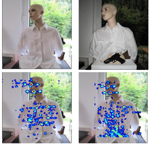
Figure 10 Upper row shows the measured sample and the hidden object. Lower row left inset show the measured data without hidden object, right inset shows with hidden object measured with the NVA design
