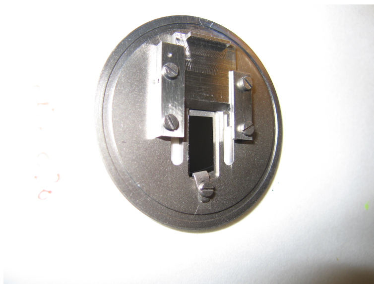
Figure 3.17: Picture of the modified sample holder. By use of the wobble stick in the deposition chamber the shutter can be pushed or pulled in-situ.
