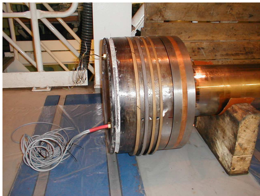
Figure 14.5: Piston before installation
