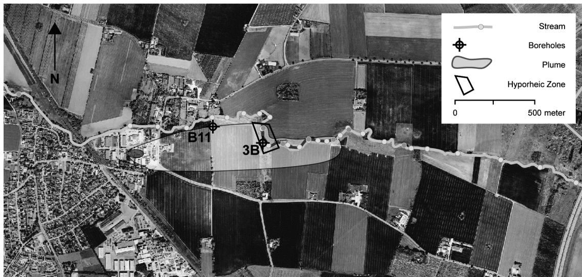
Fig. 1 Propagation of the TCE contaminant plume at the Skensved site (McKnight et al., 2010).
