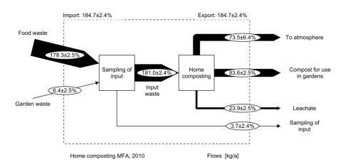
Figure 2: Material flow analysis of the home composting system in Unit 1. All numbers are in kg material yr<sup>-1</sup> based on wet weight.
