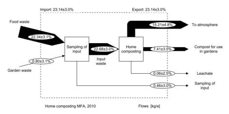
Figure 3: Substance (carbon) flow analysis of the home composting system in Unit 1. All numbers are in kg C yr<sup>-1</sup> based on dry weight.
