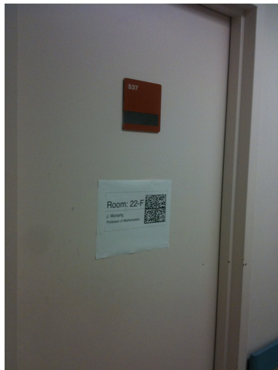
Figure 23, Doorplate design that incorporates Semantic Barcodes. These barcodes are so-called 'v-cards', that can carry a wide range of information, such as e-mail address, phone number, calendar information, website link.
