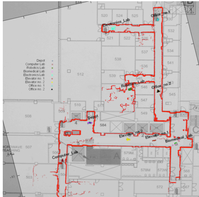
Figure 63, Generated map is overlaid on the architectural floor plan of the environment for comparison.
