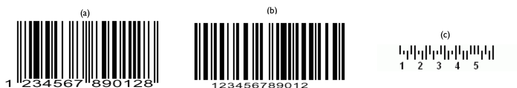
Figure 46, examples of one dimensional barcodes: (a) EAN, (b) Code 128, (c) Postnet / Royalmail
