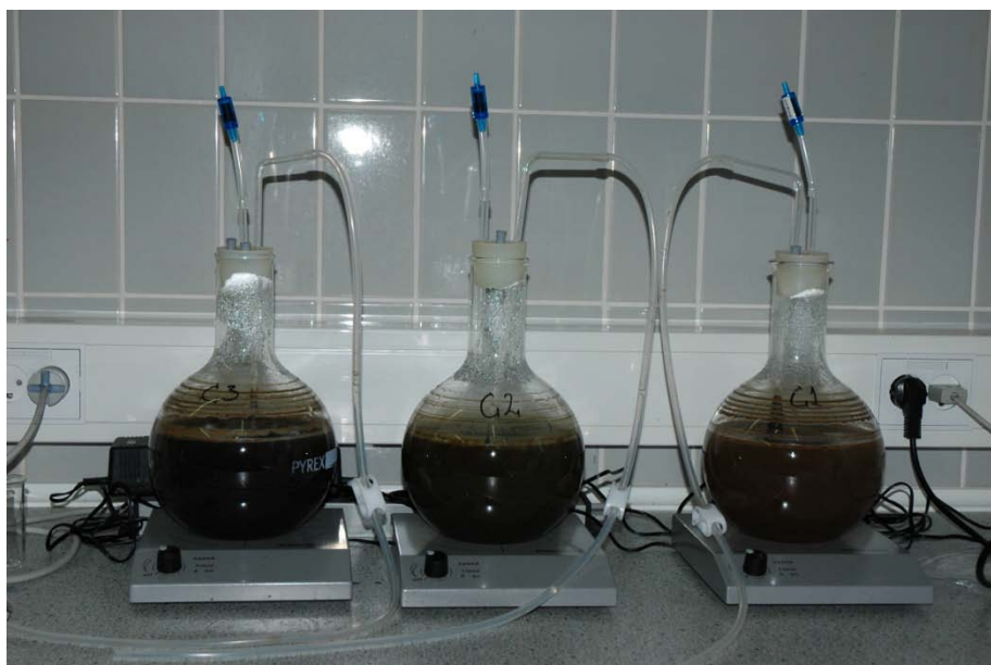
Figur 9.1. Slamhydrolyseopstilling. Slam fra biofilterskyl hydrolyseres anaerobt under omrøring.
