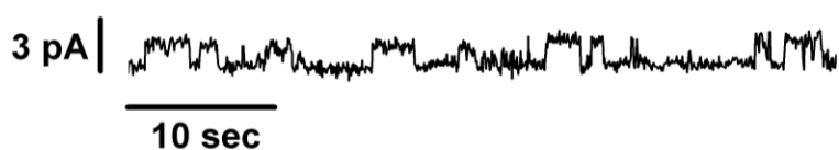
Figure 20. Single channel gramicidin current trace from an X1000P-encapsulated 5 day old DPhPE-A membrane in buffer adjusted to 1M KCl. A 60mV DC potential was applied across the membrane and the signal filtered at 10 Hz. Figure from 67 .
