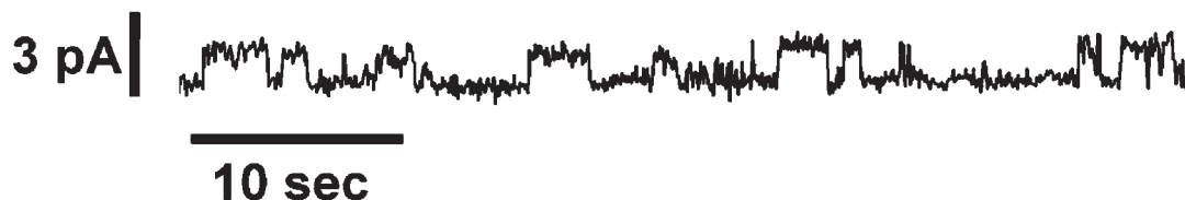
Figure 6. Single channel gramicidin current trace from an X1000P-encapsulated 5 day old DPhPE-A membrane in buffer adjusted to 1 M KCl. A 60 mV DC potential was applied across the membrane and the signal was filtered at 10 Hz.
