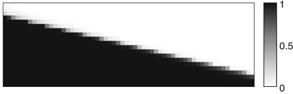
Fig. 5 Illustration of a castable field \tilde{\rho} = \mathcal{H}(\rho(y)) on a 60 \times 20 mesh with \beta = 30 , \rho = (0, 1/19, 2/19, \dots, 1)^T , a = 1.2 , b = 0.2
