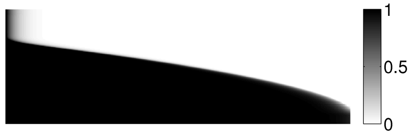
Figure 8.5 Optimized design for the MBB problem subject to a 50% volume constraint and the parameterization \tilde{\rho} = \mathcal{F}(\mathcal{H}(\rho)) cf. equation (8.5). The value of \tilde{\rho} is displayed in the graybar. Continuation on \beta = \{15, 30, 35, 40\} is performed. 480 \times 160 elements obtained in 34 iterations with c = 6.15 \cdot 10^2 . The constraint g is negative and of the order 10^{-5} - 10^{-4} .
