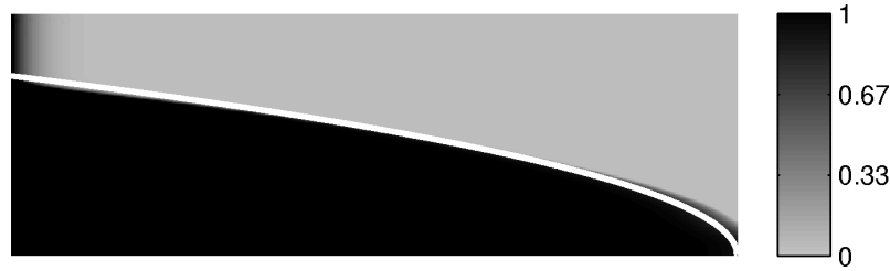
Figure 8.6 Comparison of the design in figure 8.5 with an analytic estimate of the height (white line) given by h(x) = 0.43\sqrt{L_x - x} . The estimate is obtained using Bernoulli-Euler beam theory (Pedersen and Pedersen, 2009) and a surprisingly good agreement with the design is observed despite the aspect ratio of L_x/L_y = 3 .
