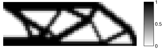
Figure 8.2 Optimized topology design for the MBB problem on a 60 \times 20 mesh with a volume constraint of 50%, the density filter with radius 1.4 element side length. The graybar shows the value of the physical density \tilde{\rho} , c = 2.16 \cdot 10^2 .
