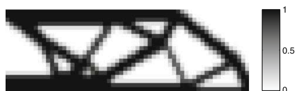
Fig. 2 Optimized topology design for the MBB problem on a 60 \times 20 mesh with a volume constraint of 50%, density filter with radius r = 1.4/20 and fixed p = 3 . The graybar shows the value of the physical density \tilde{\rho} , c = 2.16 \cdot 10^2 , g = -8.15 \cdot 10^{-6} and the design is obtained in j = 232 iterations. m = n = N = 1,200
