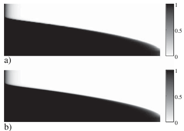
Fig. 7 Optimized design for the MBB problem subject to a 50% volume constraint and the parameterization \tilde{\rho} = \mathcal{H}(\rho) (cf. (11)). The value of \tilde{\rho} is displayed in the graybar. Continuation on \beta = \{15, 30, 35, 40\} is performed. a 240 \times 80 elements obtained in 34 iterations with c = 6.12 \cdot 10^2 and b 480 \times 160 elements obtained in 34 iterations with c = 6.15 \cdot 10^2 . The constraint g is negative and of the order 10^{-5} - 10^{-4}
