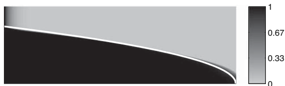
Fig. 8 Comparison of the design in Fig. 7b with an analytic estimate of the height ( white line ) given by h(x) = 0.43\sqrt{L_x - x} . The estimate is obtained using Bernoulli–Euler beam theory (Pedersen and Pedersen 2009) and a surprisingly good agreement with the design is observed despite the aspect ratio of L_x/L_y = 3 . See the Pedersen and Pedersen (2009) for further details on analytical solutions also using Timoshenko beam theory
