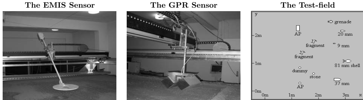
Figure 1. The artificial UXO- and landmine-field, and sensor setup. Picture to the left: The GEM-3 EMIS sensor mounted in the 2D-scanner. Picture in the middle: The bow-tie GPR antenna mounted in the 2D-scanner. Sketch to the right: The test-field setup.
