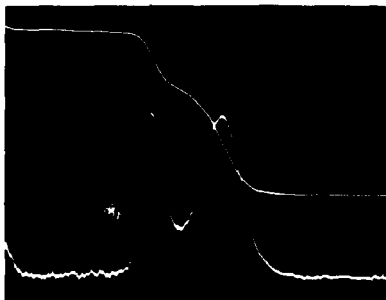
FIGURE 4: SIGNAL OF ENERGY ANALYZER. TOP TRACE IS CURRENT VS VOLTAGE. BOTTOM TRACE IS THE DERIVATIVE OF THE CURRENT VS VOLTAGE OR THE DISTRIBUTION FUNCTION. HORIZONTAL SCALE 1 V/CM.
